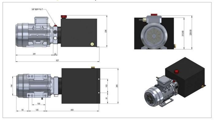
Motor: 2.2Kw 3PH 415v 1450rpm
